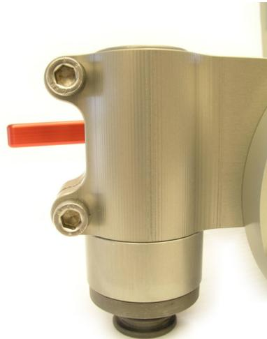
Figure 17 – Idler Shaft Clamp Bolts
