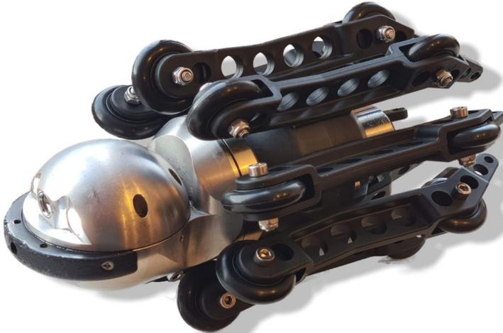
Fig. 48 - Pan and tilt camera
