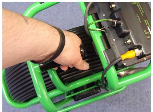
Fig. 21 - Apply brake
