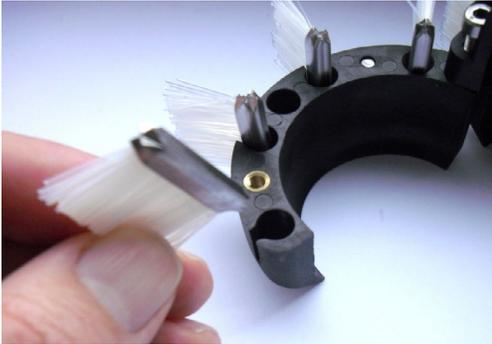
Fig. 13 - Unscrew skid and install nylon brushes
