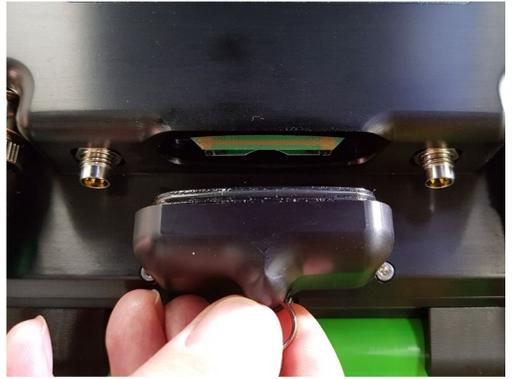
Fig. 4 - Remove SD card cover
