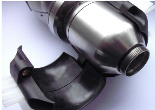
Fig. 15 - Place pushrod adapter inside skid
