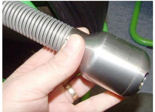
Fig. 2 - Attach camera
