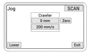
Fig. 34 - Jog screen with actuated probe lift toggle button
