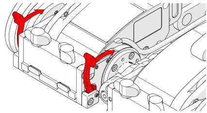
Fig. 16 - Lock swivel mount adjustment levers
