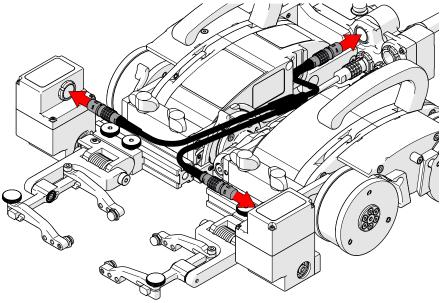
Fig. 31 - Connect split auxiliary cable
