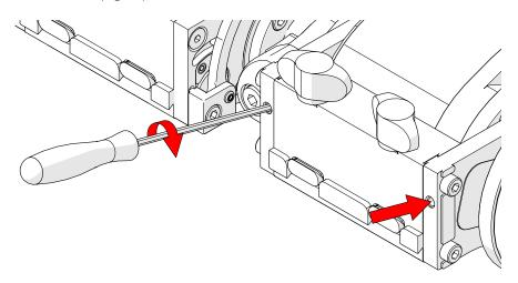
Fig. 26 - Tighten the set screws of the swivel mount.
