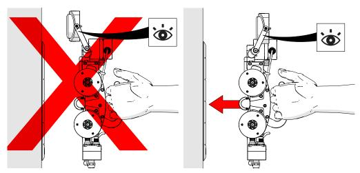
Fig. 32 - Incorrect actuated probe lift position for installation
