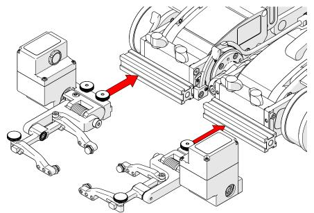
Fig. 29 - Attach actuated probe lifts
