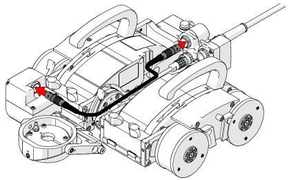
Fig. 19 - Connect auxiliary cable
