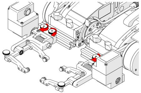
Fig. 30 - Attach actuated probe lifts
