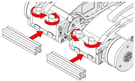
Fig. 27 - Mount frame bars to the swivel mounts
