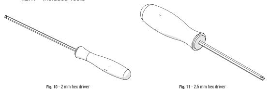
The Actuated Probe Lifts include a 2 mm hex driver (Fig. 10). This driver is used to tighten the swivel mount of the  $\bf NAVIC$ .
