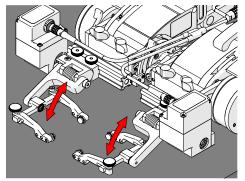
Fig. 36 - Lower/Lift actuated probe lifts
