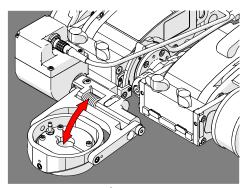
Fig. 35 - Lower/Lift actuated probe lift
