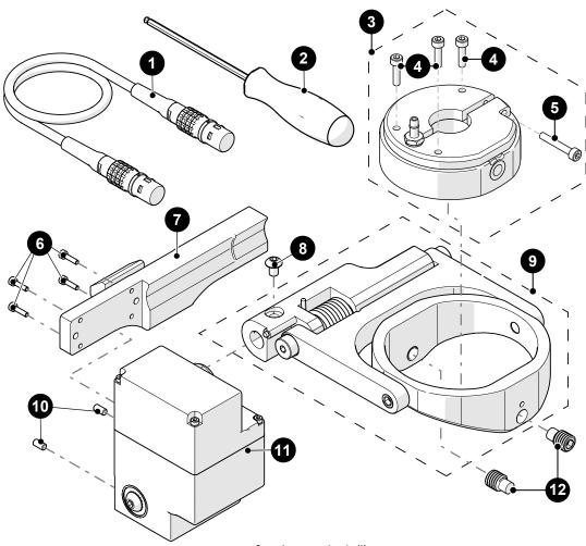
Fig. 37 - Corrosion actuated probe lift
