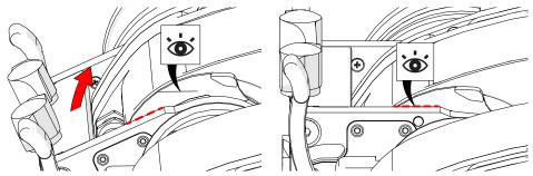
Fig. 14 - Align swivel mount with horizontal etched line
