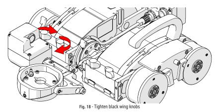
**7.** Tighten the two black wing knobs to affix the actuated probe lift to the crawler (Fig. 18).
