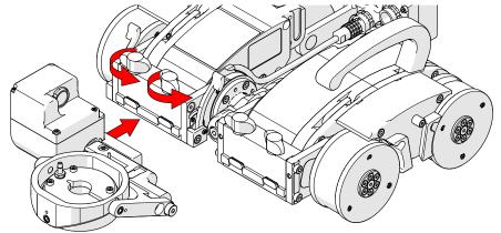
Fig. 17 - Loosen black wing knobs and mount to crawler
