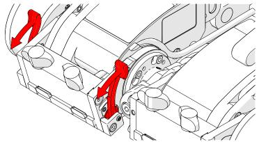
Fig. 21 - Release swivel mount adjustment levers
