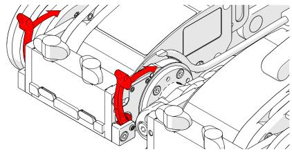
Fig. 24 - Lock swivel mount adjustment levers
