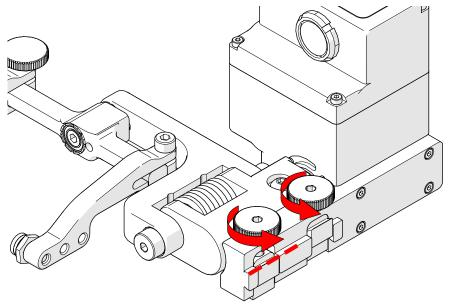
Fig. 28 - Loosen probe holder adjustment knobs
