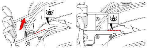
Fig. 22 - Align swivel mount with horizontal etched line
