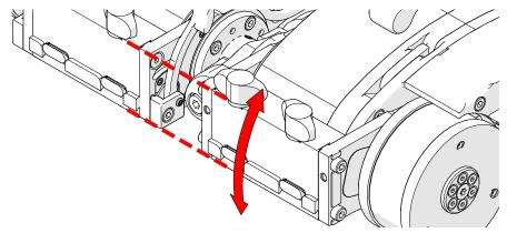
Fig. 25 - Align left swivel mount with right swivel mount
