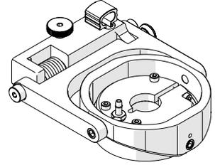
Fig. 33 - Corrosion thickness probe holder
