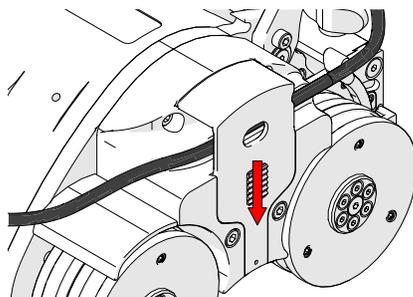
Fig. 98 - Place cables and hoses then close retainer
