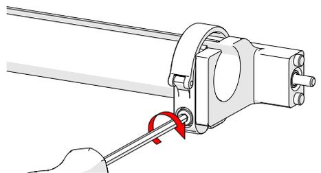
Fig. 206 - Tighten clamp screw
