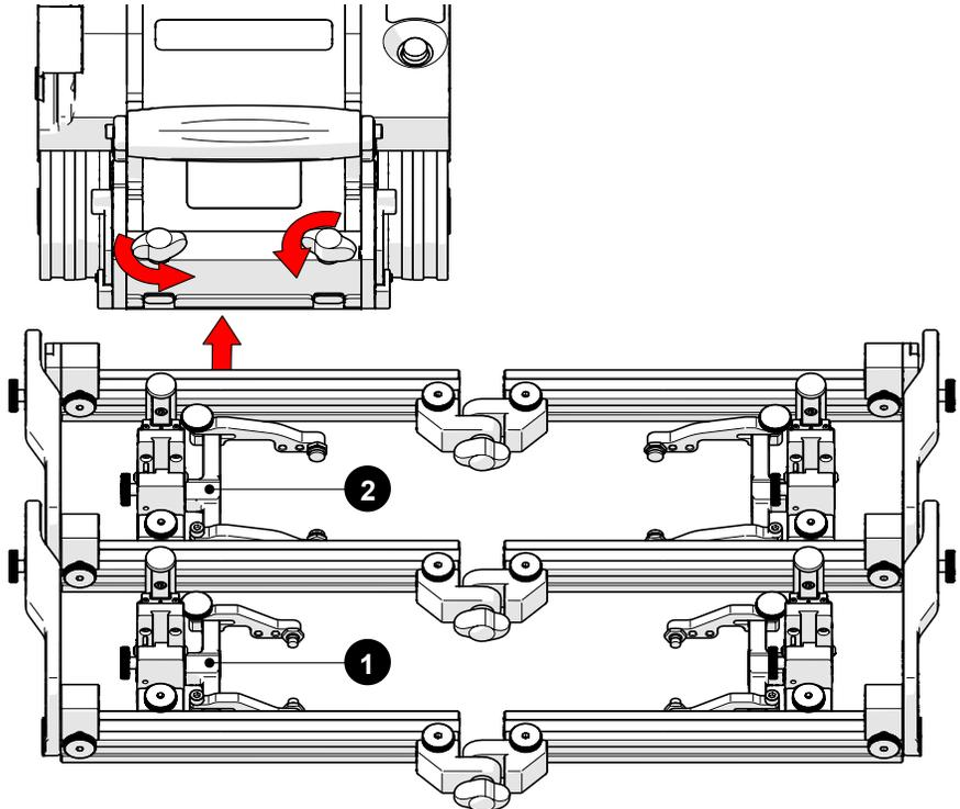
Fig. 185 - Connect frame to crawler's swivel mount
