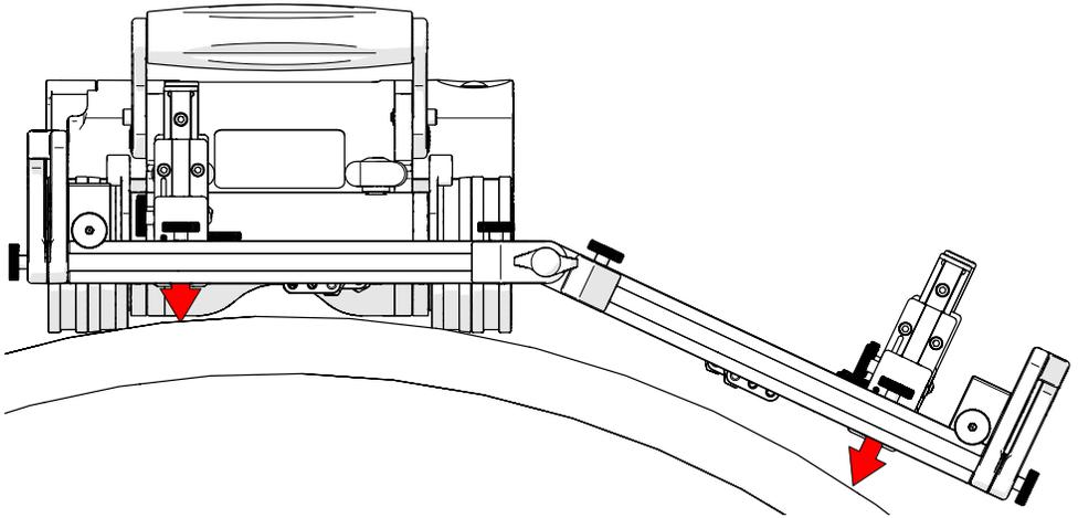
Fig. 187 - Tighten pivot wing knobs
