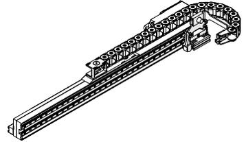
Fig. 74 - Motorized raster arm
