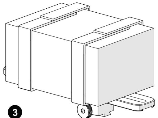
Fig. 209 - Mount bracket on a frame bar
