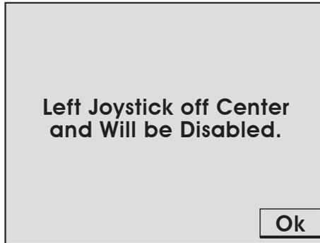
Fig. 238 - Joystick off centre screen
