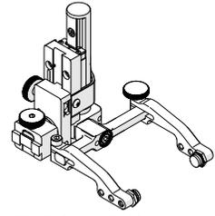
Fig. 30 - Vertical probe holder
