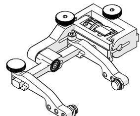
Fig. 64 - Slip joint probe holder
