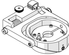
Fig. 32 - Corrosion thickness probe holder
