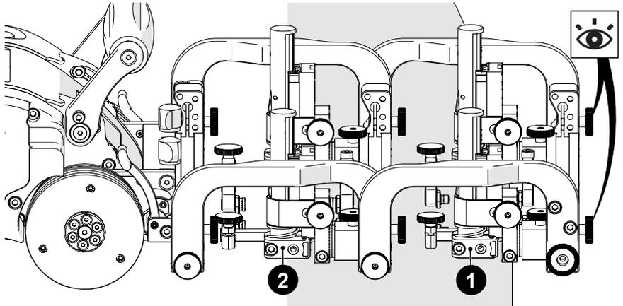
Fig. 178 - Position primary and secondary probe holders
