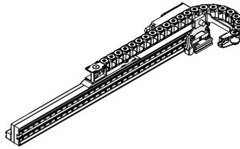
Fig. 40 - Motorized raster arm
