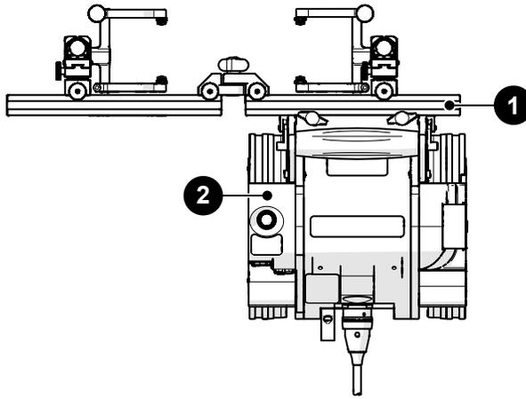
Fig. 83 - Pivoting probe holder frame configured for flange scanning
