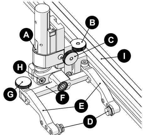
Fig. 122 - Vertical probe holder
