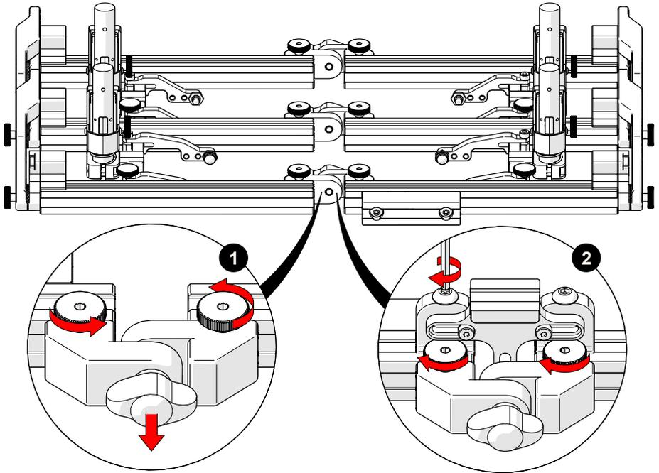
Fig. 193 - Correct probe holder longitudinal adjustment
