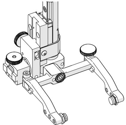
Fig. 146 - Reversed probe holder
