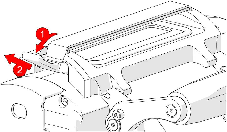
Fig. 103 - Press lever down and pull to release
