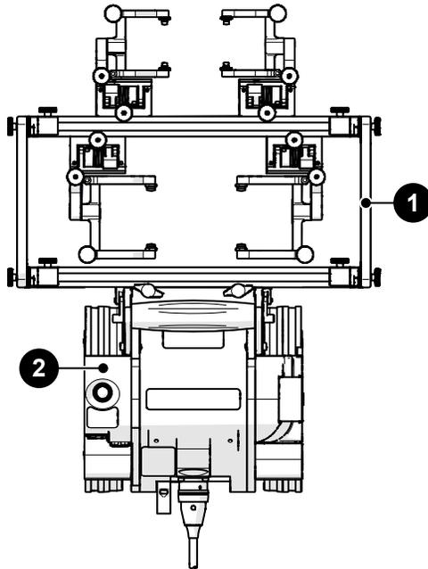
Fig. 81 - Low profile probe holder frame configuration
