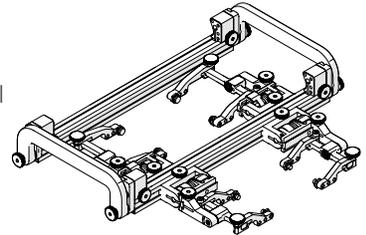
Fig. 60 - Low profile probe holder frame
