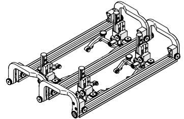
Fig. 61 - Vertical probe holder frame
