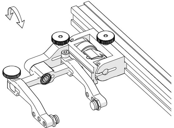
Fig. 170 - Reversed probe holder
