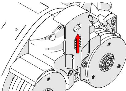
Fig. 97 - Lift retainer by hand
