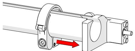
Fig. 205 - Slide clamp onto mount
