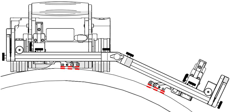
Fig. 188 - Correct probe holder longitudinal adjustment
