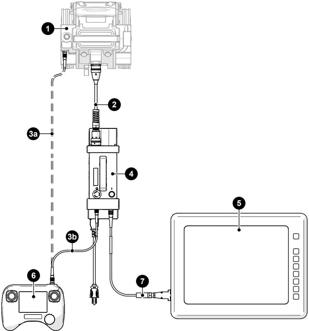
Fig. 79 - Standard crawler configuration
