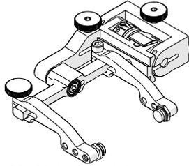
Fig. 29 - Slip joint probe holder
