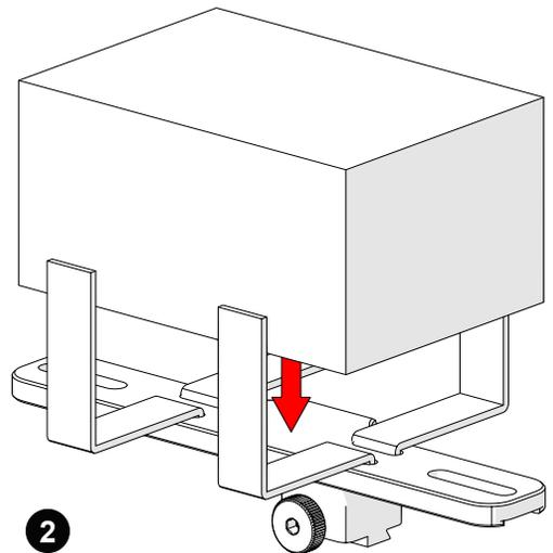
Fig. 208 - Place preamp and wrap velcro
