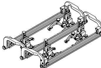
Fig. 26 - Vertical probe holder
