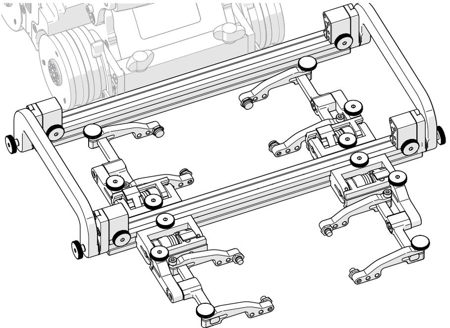
Fig. 171 - Low profile probe holder frame
