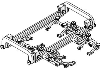
Fig. 25 - Low profile probe holder frame
