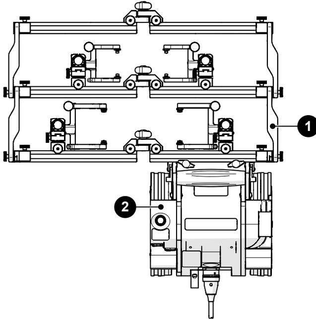
Fig. 82 - Pivoting probe holder frame configuration
