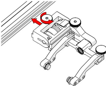
Fig. 148 - Attach to frame bar
