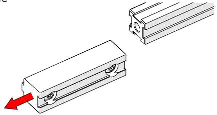
Fig. 184 - Remove probe holder pivot mount
